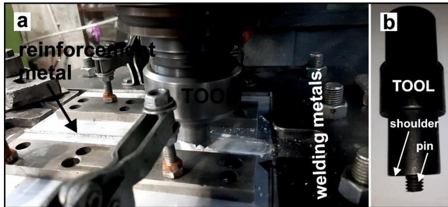
Figure 1. The FSW experimental layout (a) and tool used in FSW applications (b)
